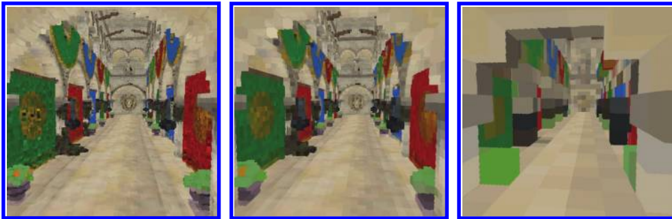
Figure 22.10. The Sponza scene voxelized into our octree structure at a maximum resolution of respectively 512^3 , 256^3 , and 64^3 voxels and rendered without filtering.
