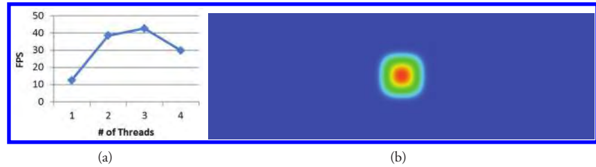
Figure 42.4. (a) Performance of parallel heat transfer. (b) Example: parallel finite difference-based heat transfer.
