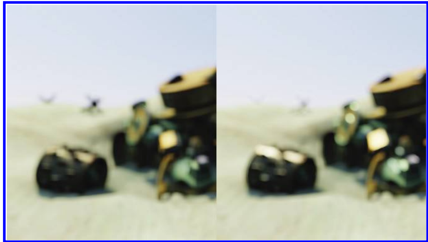
Figure 15.1. Comparison between a simple blur-based depth of field (left) and a depth of field with bokeh rendering (right).
