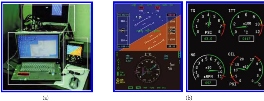
Figure 8.8. Developing on an embedded system: (a) development environment; (b) screen output.
