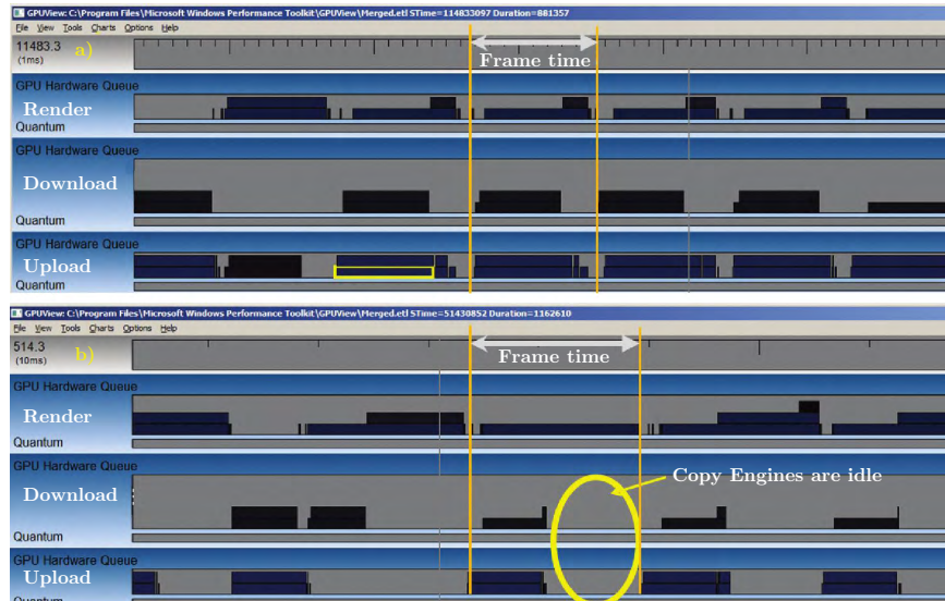
Figure 29.17. Ideal case of bidirectional transfers where upload, render, and download take the same time (top). Render-bottlenecked applications where the copy engines are idle 50% of the time (bottom).
